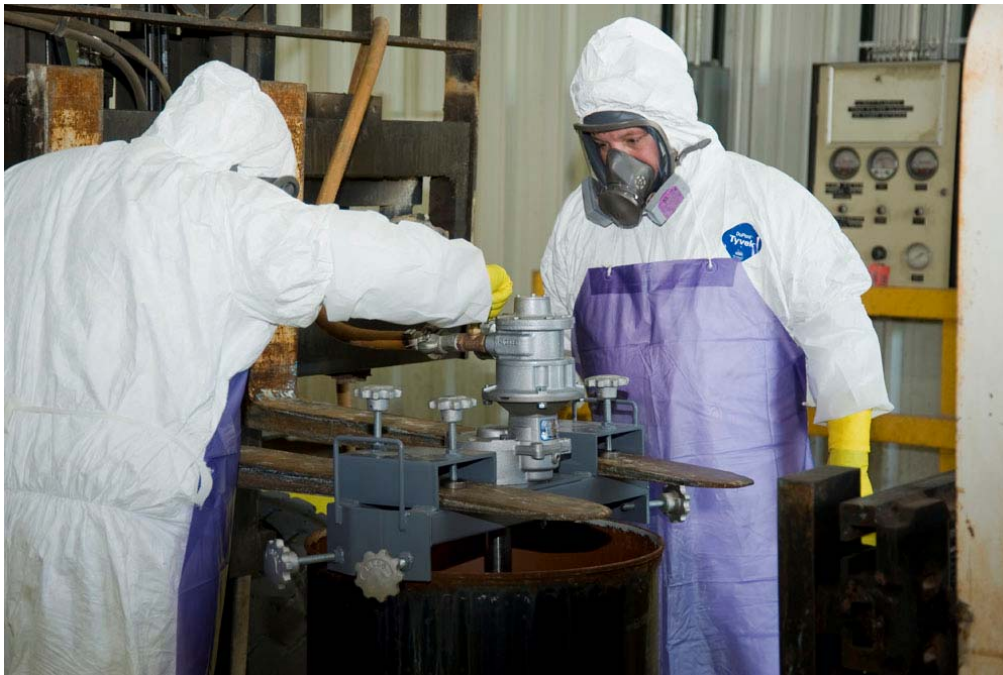
Solidification of mineral oil for Alpha 5 being performed at Y-12 facility
