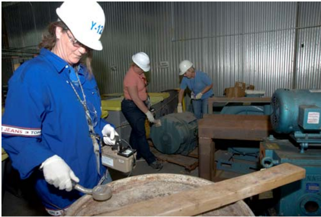
Workers executing radiological characterization of Alpha 5 materials
